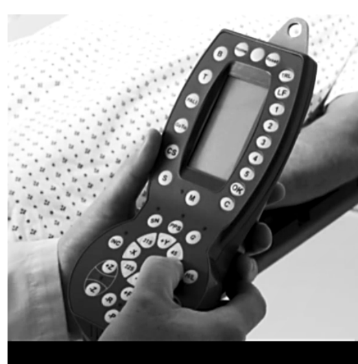
Figure 2: Teach pendant device currently used in treatment room (courtesy of IBA)
